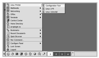
You can also access the Linux Printer Configuration window by typing in "linux-config" from the Terminal screen.
